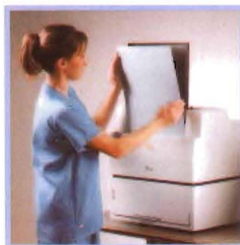
Remove the exposed storage plate from the cassette and place it in the plate reader.
