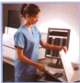
A reusable storage phosphor plate replaces film in a therapy or simulation cassette. Using standard techniques, the plate is exposed just like film.
