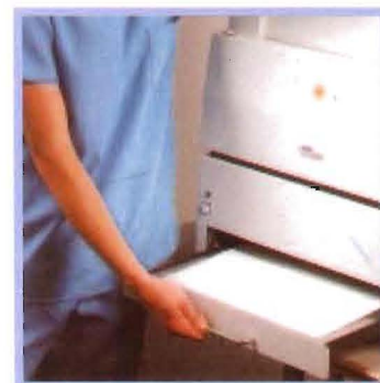
The reader scans a 2.5 MB image in 25 seconds and produces a high-quality digital image on the display. The plate is automatically erased and placed back in the cassette for reuse.
